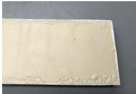
Close-up view of blisters
